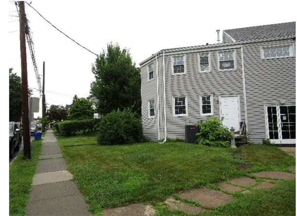
A rain garden can be installed in the turfgrass area near the downspouts of the southeast corner near the entrance of the building to capture, treat, and infiltrate stormwater runoff from the roof. Two other rain gardens can be installed along the west end of the building by redirecting downspouts into the gardens. A preliminary soil assessment suggests that more soil testing would be required before determining the soil's suitability for green infrastructure.
