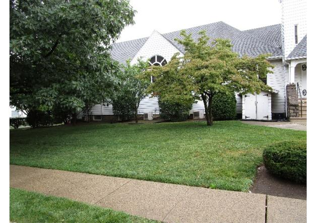
Parking spaces can be converted to porous pavement to capture and infiltrate stormwater runoff from the parking lot. Rain gardens can be installed in the turfgrass areas at the eastern side of the building to capture, treat, and infiltrate stormwater runoff from the roof if the downspouts are disconnected. A preliminary soil assessment suggests that the soils have suitable drainage characteristics for green infrastructure.
