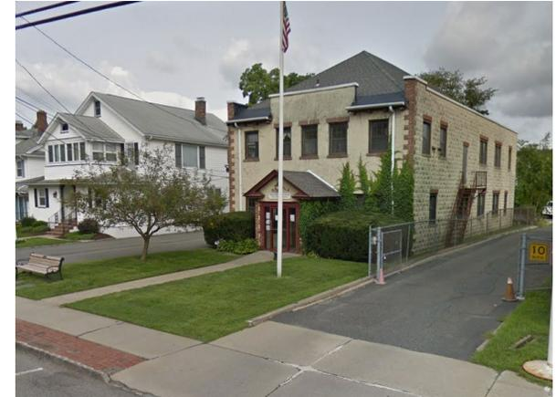
A rain garden can be installed at the front of the building around the flag pole by disconnecting the downspout from the corner of the building into the garden. A preliminary soil assessment suggests that the soils have suitable drainage characteristics for green infrastructure.
