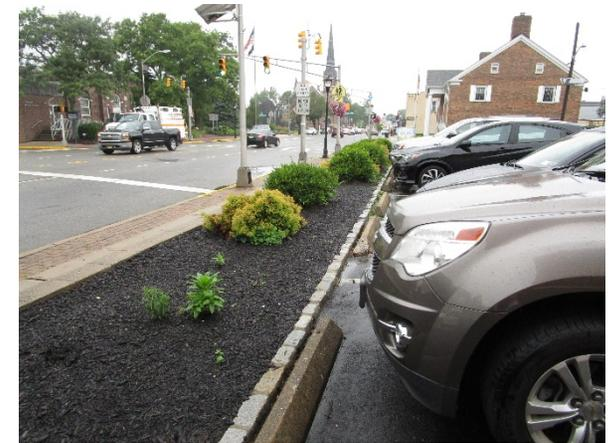
A rain garden can be installed in the turfgrass and shrub area along the side of the building to capture, treat, and infiltrate stormwater runoff from the roof. Parking spaces in the parking lot can be converted to porous pavement to capture and infiltrate stormwater runoff from the front parking lot. A preliminary soil assessment suggests that more soil testing would be required before determining the soil's suitability for green infrastructure.
