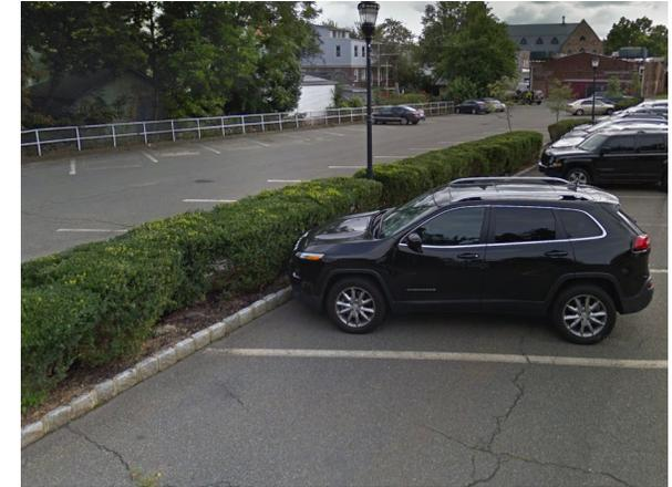
Parking spaces throughout the lot can be converted to porous pavement to capture and infiltrate stormwater runoff from the rest of the parking lot. A preliminary soil assessment suggests that more soil testing would be required before determining the soil's suitability for green infrastructure.
