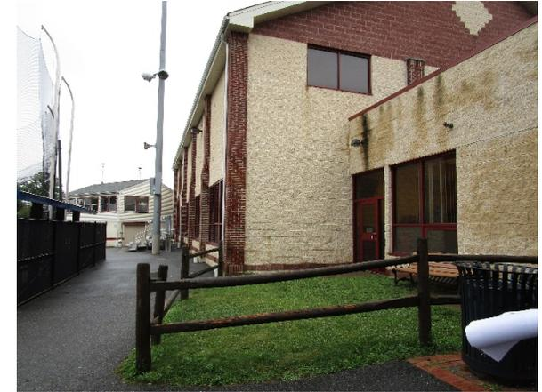
Several rain gardens can be installed in the turfgrass area around the municipal complex to capture, treat, and infiltrate stormwater runoff from the field and help reported flooding in the area. A preliminary soil assessment suggests that more soil testing would be required before determining the soil's suitability for green infrastructure.
